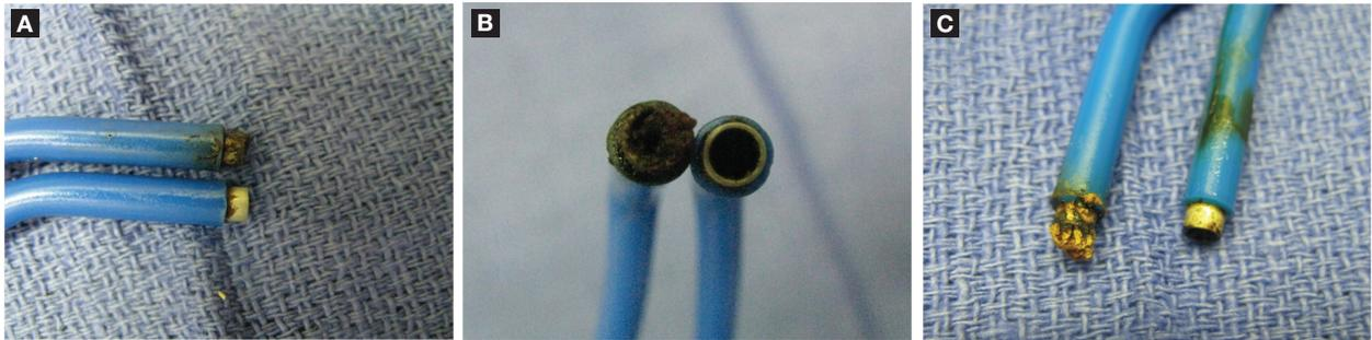
Figure. **A:** Photo shows two suction cautery tips after 30 seconds of cauterizing bovine renal tissue. The instrument on the bottom is coated with Electro Lube. **B:** Another photo shows two other tips after 30 seconds. The coated tip is on the right. **C:** Tips are seen after 60 seconds of cauterizing. The coated instrument is on the right.
